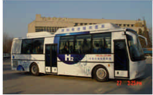
FIG. 1. Photo of the fuel cell city bus developed.
